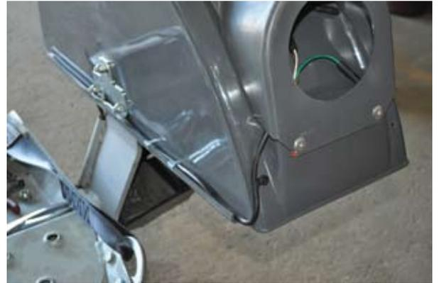
15. Push wires back into housing and finish routing wires in wire trough of fender and attach cable hanger. With pliers install two metal wire clips. Place one clip 5-1/2" from rear of fender and one 8" from rear of fender.
