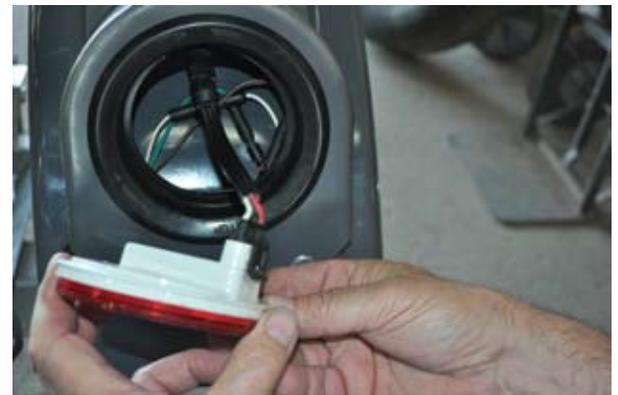
16. Install rubber grommet and attach 3-wire pigtail harness to fender wiring. Coil pigtail harness inside of fender housing and plug into 4" round LED light. Push light into grommet.
