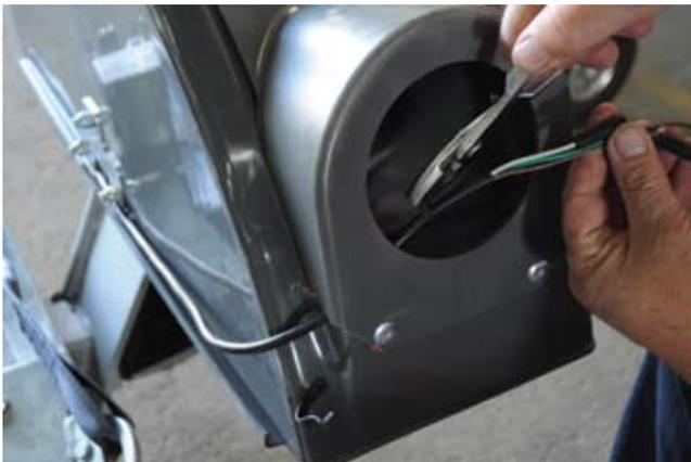
14. Pull all wire from light hole in housing and install the snapper hose clip approximately 1-1/2" back from end of wire shielding. Squeeze snapper clip tight with pliers.
